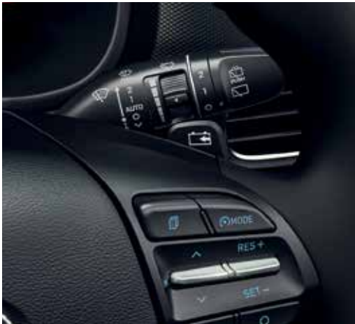
Paddle shifter (regenerative braking control)
